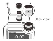
1.4 Press the **Meas** key, the meter begins measurement, the <sup>(c□)</sup> icon shows on the screen. When the reading stabilizes, the icon will automatically switch to □.
