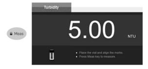
1.5 If necessary, press the **Meas** key to take a new measurement.
